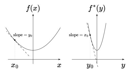
Assume that f is a closed and convex function. Then f is strongly convex with parameter  $\mu \Leftrightarrow \nabla f^*$  is Lipschitz with parameter  $1/\mu$ .
