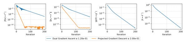
We need to find a minimum of a quadratic function in some linear subspace, defined by the solution of linear equation Cx = d. This is a conditional optimization problem, we start from strongly convex setting.
