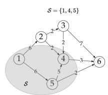
The edges in the cut are  $1\to 2, 4\to 6$ , and  $5\to 6$  the capacity of this cut is 6+3+2=11.
