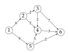
The nodes are routers, the edges are communications links; associated with each node is a capacity — node 1 can communicate to node 2 at as much as 6 Mbps, node 2 can communicate to node 4 at upto 2 Mbps, etc.
