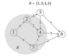
The edges in the cut are  $2 \rightarrow 3, 4 \rightarrow 6$ , and  $5 \rightarrow 6$  the capacity of this cut is 2+3+2=7.
